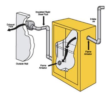
The above NFPA guidelines refer specifically to flammable liquid storage cabinets; if, at the request of your AHJ, you're required to vent a corrosives/acid cabinet, make sure to incorporate a blower that's compatible with the vapors being exhausted. Also be aware that if it's a hazardous material you're venting, you may not be allowed to exhaust to the outside due to the health hazards the vapors present.
