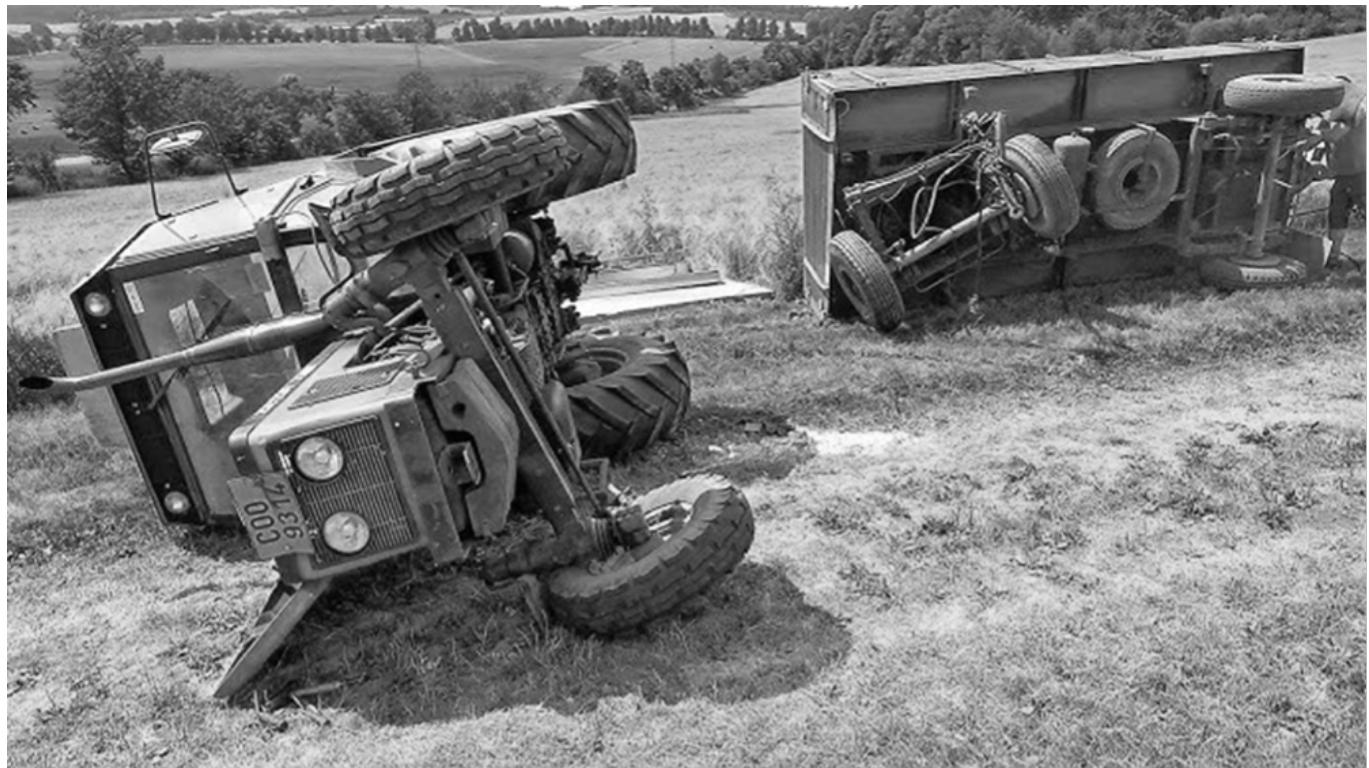
The overturned tractor and trailer suggest a hitching failure or improper load balance during operation. This indicates the hitch was either not secured correctly or the terrain and slope were not adequately assessed beforehand. Such rollover incidents pose serious risks of injury or death to the operator and damage to equipment.
