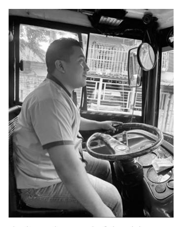
The image shows a school bus driver operating the vehicle without wearing a seat belt. Seat belts are a critical safety requirement for drivers, as they provide protection in the event of a sudden stop, collision, or loss of control. Additionally, the driver's posture appears somewhat relaxed. Proper driver posture is essential for maintaining full control of the vehicle and reacting quickly to potential road hazards.
