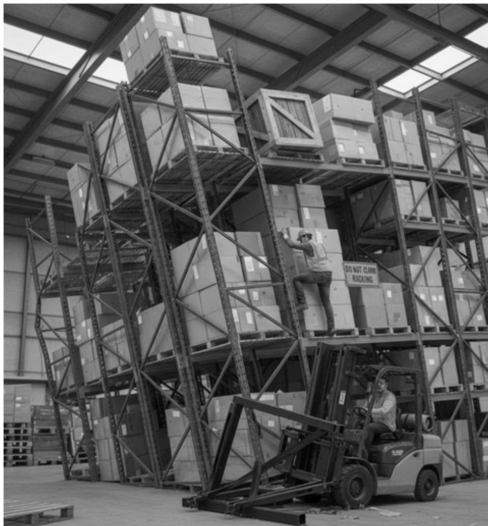
This image shows a worker climbing warehouse racking, directly beside a sign that says "**DO NOT CLIMB RACKING.**" This is a serious violation of safe storage and inspection practices. The racking is visibly overloaded and misaligned, posing risks of collapse, falling objects, and serious injury. Additionally, a forklift is operating directly beneath the worker, an extremely unsafe overlap of pedestrian and equipment zones.
