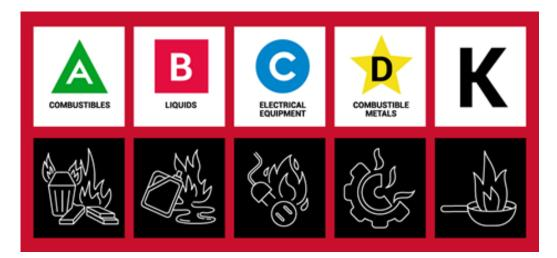
Class A fire extinguishers are used for ordinary combustibles such as wood, paper, some plastics and textiles. This fire class requires the heat-absorbing effects of water or the coating effects of certain dry chemicals. According to NFPA, extinguishers suitable for Class A fires should be identified by a triangle containing the letter "A." If in color, the triangle should be green.
