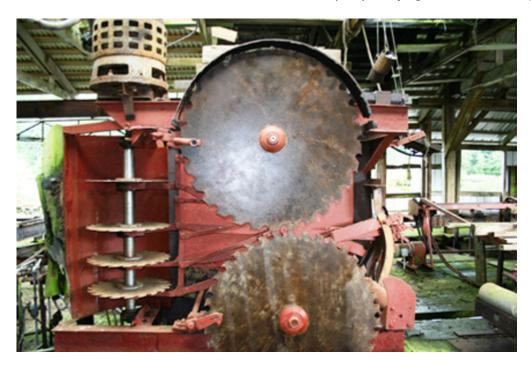
These brutes are seven-foot saws in a double circular mill arrangement. And they're not properly guarded.
