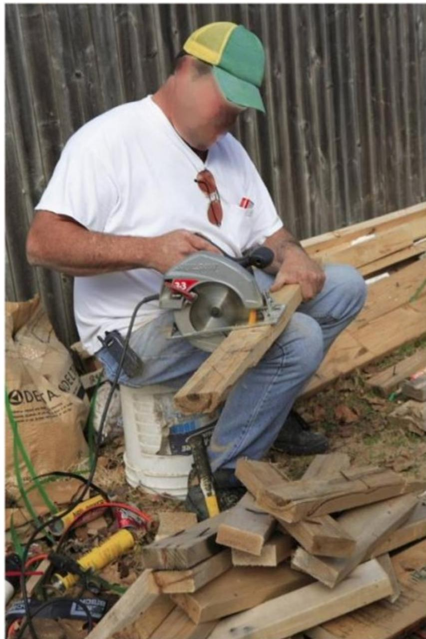
Of all the dangerous things the worker operating this handheld circular saw is doing, the one that scares me the most is using his legs to brace the board he's cutting.
