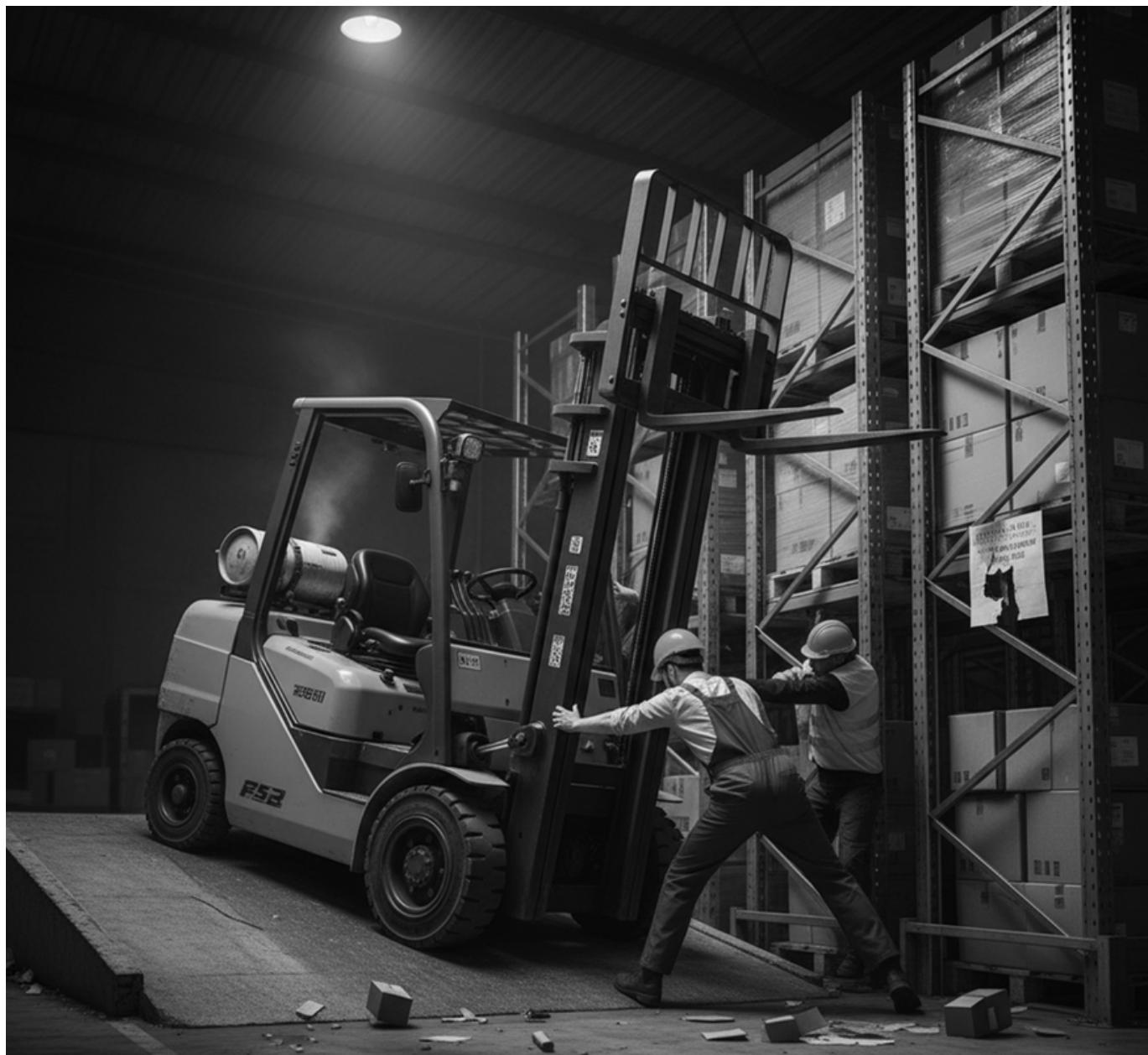
This image shows a forklift parked improperly on a ramp or incline, with the forks elevated and workers dangerously close to the equipment. One worker is physically touching the forks, and another is standing in the fall zone.
